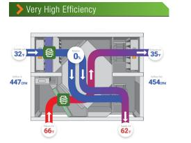
Every Ventacity ventilation unit offers industry-leading efficiency, controls, and energy savings. In VS1000 RTh actual performance 1/26/2022 shown here, when the outside air is 32F the incoming 100% fresh air is already 62F after passing through the HRV—this is the source of robust energy savings.
